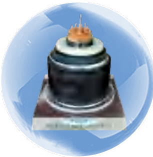
220kV Copper Conductor XLPE Insulated Corrugated Aluminum Sheathed Flame-retardant Sheathed Power Cable
