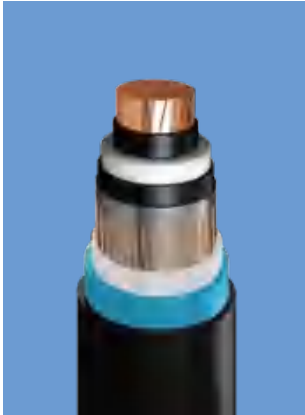
500kV XLPE Insulated Copper Wire Screen Aluminum Plastic Tape Power Cable
