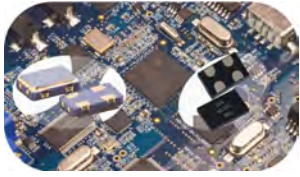
MEMS Oscillator can be Pin-to-Pin quartz Oscillator
