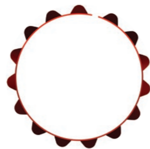
Standard SV ring in free state condition (small gap or overlap)
