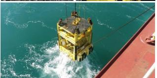
The Manta-200 is Geomil Equipment's most capable Cone Penetration Testing (CPT) system for seabed operations. Since its introduction in 2013 it has successfully completed challenging projects around the world and its performance is unsurpassed.
