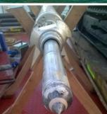
The Orca-90 is Geomil Equipment's versatile and fully integrated Cone Penetration Testing (CPT) testing and sampling system for downhole use and is designed to be combined with several existing drilling methods.
