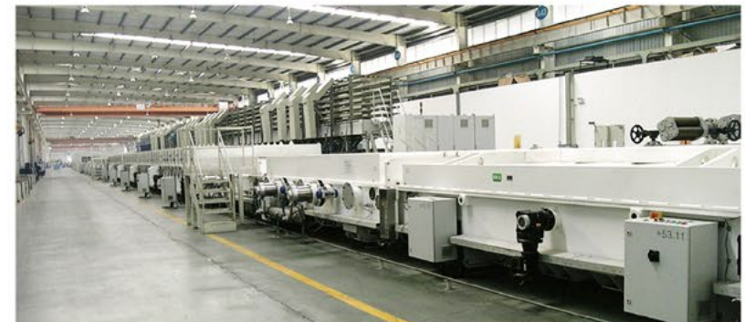
Magnetron Sputtering Coating Line with 50 cathodes
