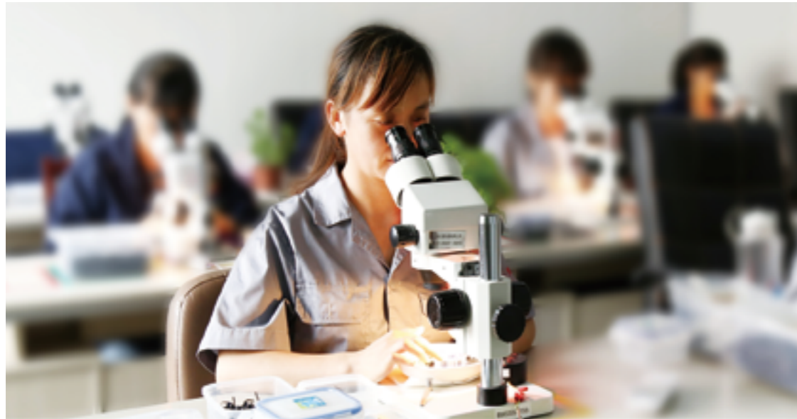
连续变焦显微镜：检测单体陶瓷球表面缺陷 Continual zoom microscope: Detection of single ceramic ball surface defect.
