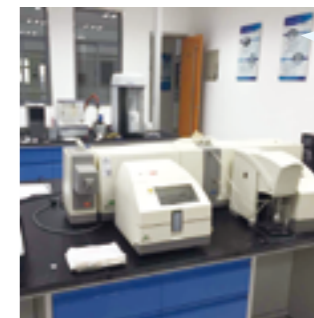
laser diffraction particle size analyser Applied for measuring size distribution of micrometer powders.
