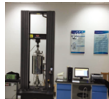
High temperature universal testing machine Applied for testing the mechanical properties of ceramics material in high temperature.
