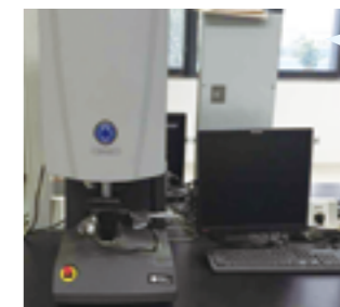
Digital micro hardness tester Applied for testing Vickers hardness of solid materials.
