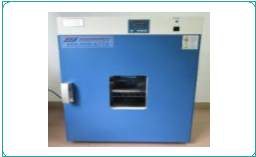
Equipment: Baking and Dry Packing Function: Baking of all PCB boards and semiconductor devices.
