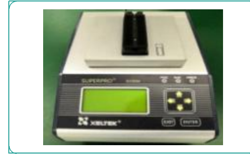
Equipment: Programming Function: Test all chips that can support programming.
