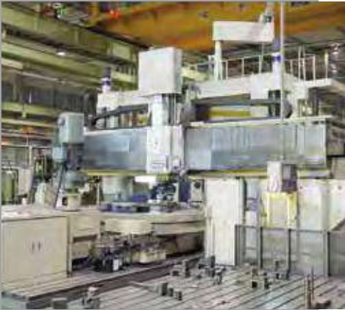
Large five-axis milling machine 大型5面加工機
