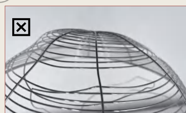
Poor Welding Joints --Easily Deformed
