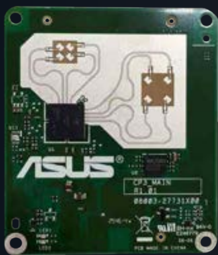
mmWave Sensor Size : 55 x 65 mm (PCBA)
