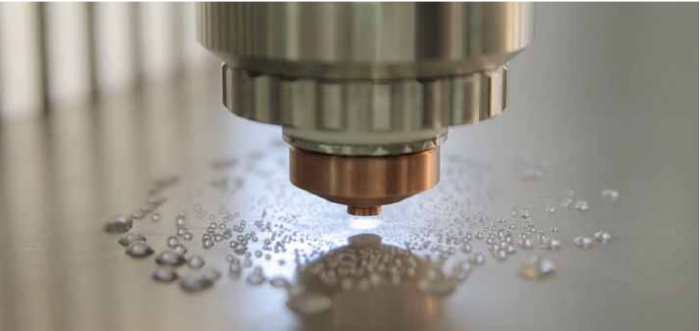
CoolTec: Ideal for permanent stable cutting of thick mild steel - due to direct water cooling of the sheet.
