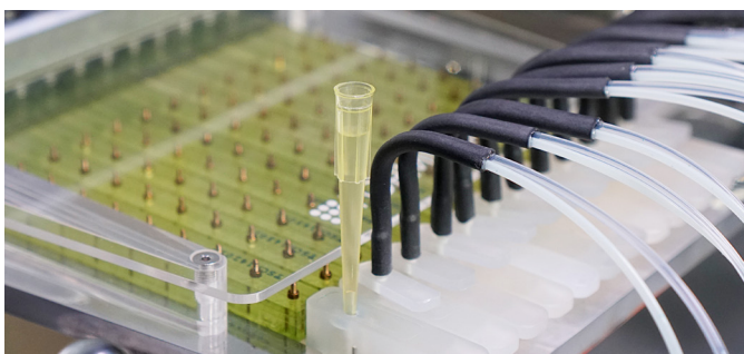
Direct pipette tip dispenses reduce dead volumes of only 100 µL
