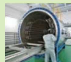
Conducting a durability test using hydrogen gas
