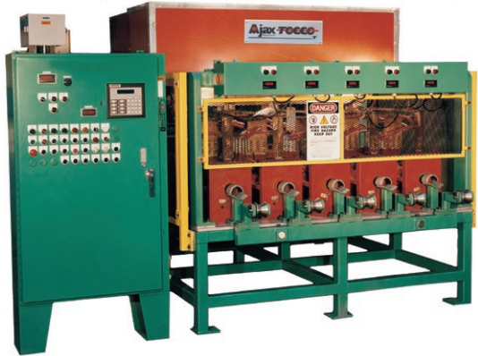
Five-position, pigeon hole style bar end heating system.
