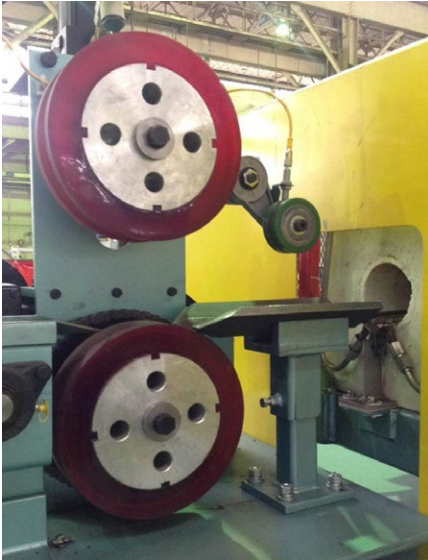
Dual powered pinch roll drive drives with standard urethane wheels or optional metal drive wheels
