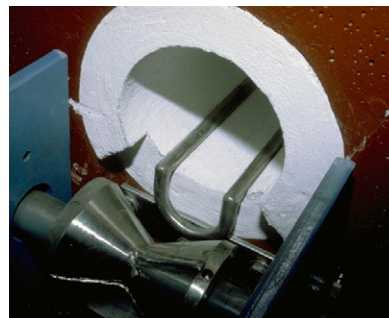
Patented wobble wheel at exit end of machine and ID of coil with hard faced coated water cooled wear rails
