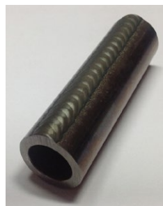
Cross Section of a Plasma Coated Hard Faced Rail
