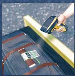
Baggage reconciliation, performed with industrial hand held readers as such as Datalogic's PowerScan imagers ensures that luggage is loaded onto the correct aircraft.
