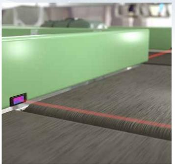
Different types of sensors such as photocells and light curtains are used in baggage handling systems for tracking, height control, and positioning. Encoders are used for conveyor speed measurement.
